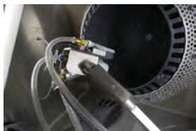
Blast gun in automatic cleaning position
