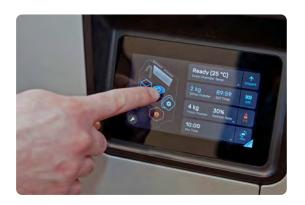
3. Ejecting the cake: Use the physical and virtual touch controls to raise and lower the print bed, allowing you to stagger the cake as it ejects from the build chamber into the Fuse Sift workspace. This is helpful for prints that contain a densely packed assortment of small or various parts.
