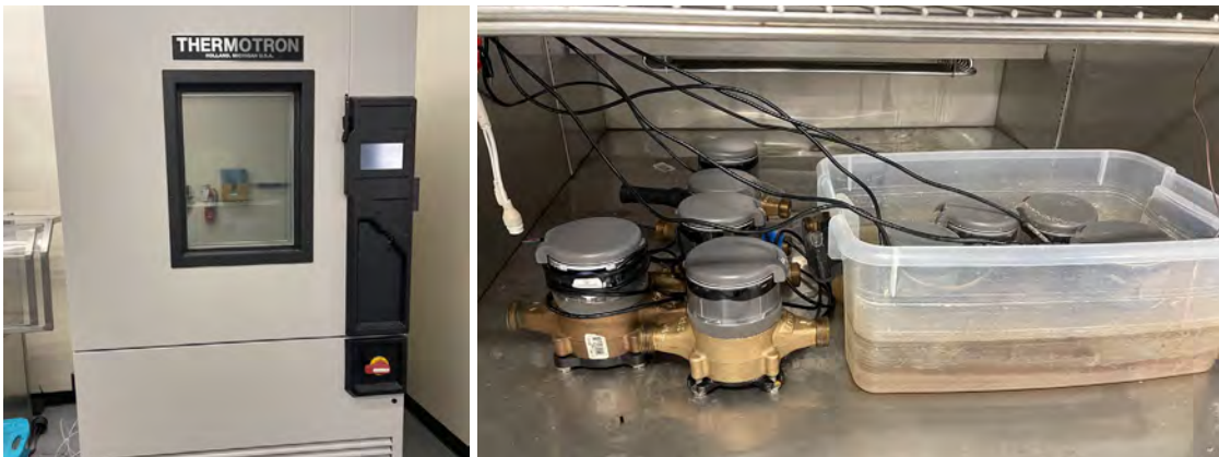
Thermotron SM environmental chamber (left) and samples installed inside (right).
