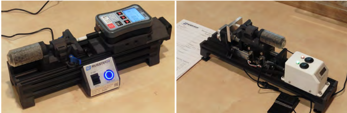
Automated Tool Tester (left) and cycle tester (right). A prototype of the contact retention tool is inserted in the testers. The tool grip is 3D printed in Elastic Resin on the Form 3 printer and will be injection molded in black TPE for the commercialized version, while the core of the tool will remain 3D printed in Nylon 12 with the Fuse 1. The tests are run using a specifically designed Delrin test probe. This specific unit is calibrated to a 6 pound force with a tolerance of \pm 0.5 pound.
