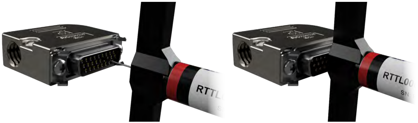
The RTTL tool inserted into a connector. The probe in the front of the tool pushes on the pins or sockets of the connector to ensure they are properly seated.
