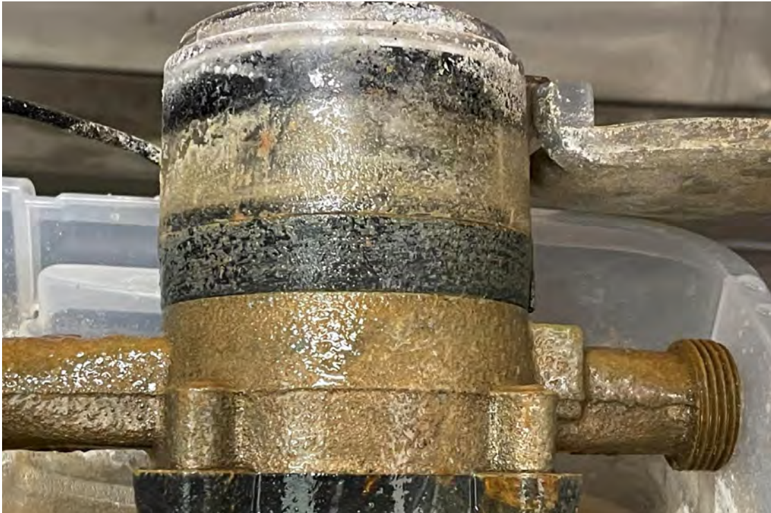
Picture of the water meter after three months testing.
