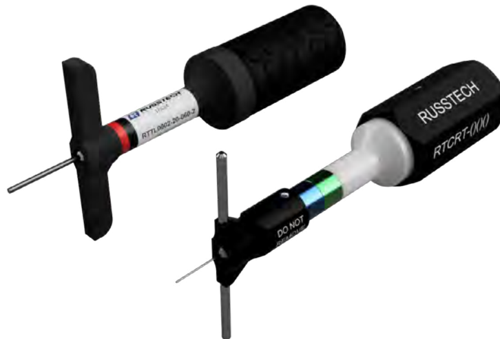
The legacy contact retention tool (right) is an assembly of multiple parts. The body is machined Delrin, the wings are machined stainless steel, and the wing stop safety feature and handle are machined aluminum. The new tool (left) is almost entirely SLS 3D printed in Nylon 12. All versions have a metallic probe at the front.
