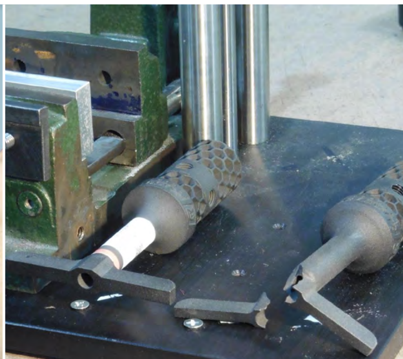
Testing the impact strength on the wing stop of the tool 3D printed in Nylon 12. The original design version broke (right) while the new design (left) survived the test.
