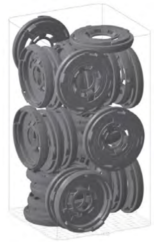
CAD model of mounting rings loaded in the PreForm print preparation software. The Fuse 1 can fit nearly 30 rings per build, with about 30 hours of printing time per job.
