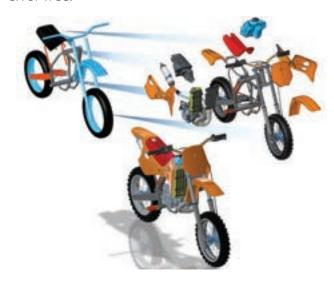
Creo AAX offers advanced assembly capabilities, such as skeleton models and data-sharing features, to support top-down design. Design criteria related to the assembly can easily be communicated to teams working concurrently on designs.
