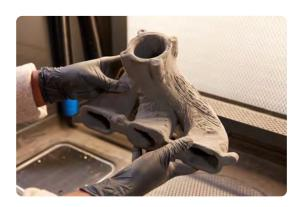
**5. Polishing:** Fuse Blast comes with the option to polish parts with a simple add-on. Simply insert the polishing system into Fuse Blast and switch your media to the Formlabs polishing media, then select a cycle or choose your custom settings.
