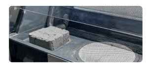
4. Extracting parts: Extract the parts from the cake of unsintered powder, breaking chunks by hand and shaking off the loose powder. When using Fuse Blast for the cleaning step, parts only need to be roughly depowdered and placed in the transfer container. This step should only take 5 minutes.
