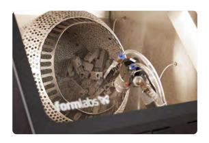
3. Manual Cleaning: For large or intricate parts, Fuse Blast comes with the option to switch to manual blasting. Simply adjust the nozzle and hold your parts with both hands under the jet, or pick up the blasting gun for handheld media blasting.
