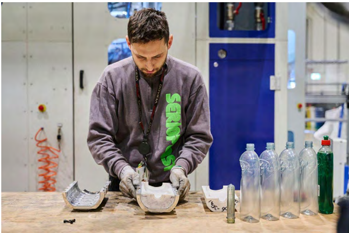
The mold 3D printed with Rigid 10K Resin is manually polished and then assembled into a metal frame.
