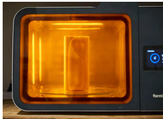
After washing, the supports are removed and the mold is post-cured.
