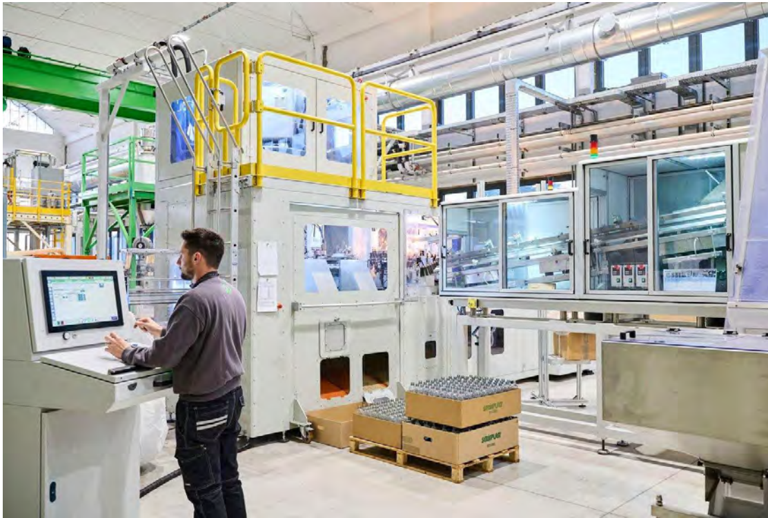
Seriomac UNIX 4 Cavities SBM machine from Serioplast in their R&D facility in Italy. Together with Unilever, they developed a new workflow for using 3D printed molds in this large-scale industrial manufacturing equipment.
