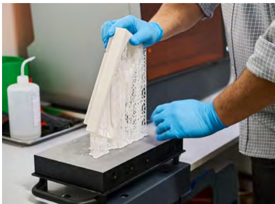
The mold is 3D printed on the Form 3L with Rigid 10K Resin.
