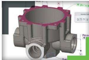
**Easier Model-based Definition (MBD) and Detailing.** A modernized symbol interface streamlines model-based definition workflows. GD&T advisor gives you enhanced support for assemblies.
