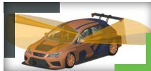
**Enhanced Ergonomics Design.** The latest enhancements to Creo allow you to account for the range of movement, the field of vision and uniqueness of users in a safe and efficient manner. The Visual Field can now perform reflection analysis and Manikins can now support multiple reach envelopes.
