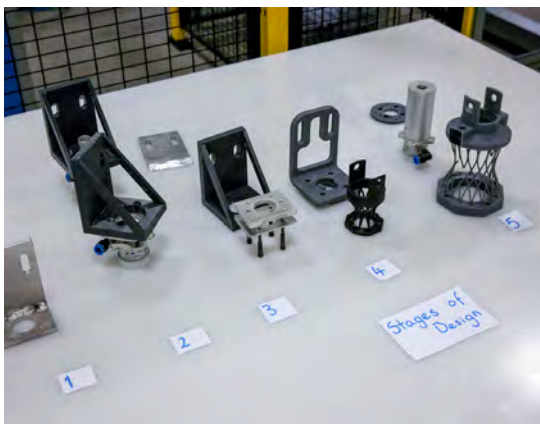
Consecutive iterations of a pick and place robot gripper prototyped on Formlabs SLA printers.
