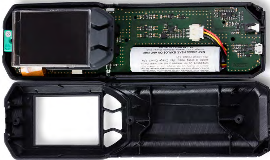
Engineers at Wöhler built a looks-like, works-like prototype of a moisture meter from multiple materials with rigid housing and soft-touch buttons.
