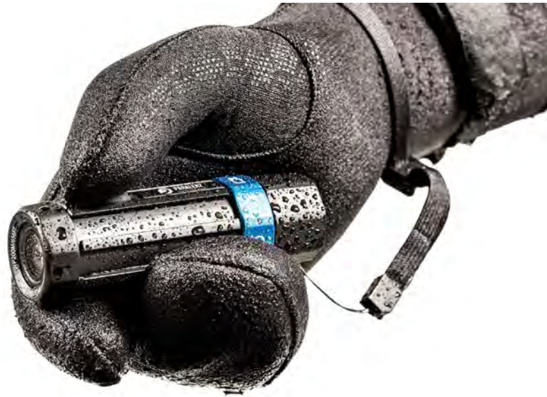
Diving camera manufacturer Paralenz used 3D printing to create functional prototypes that endured testing 200+ meters below sea level.
