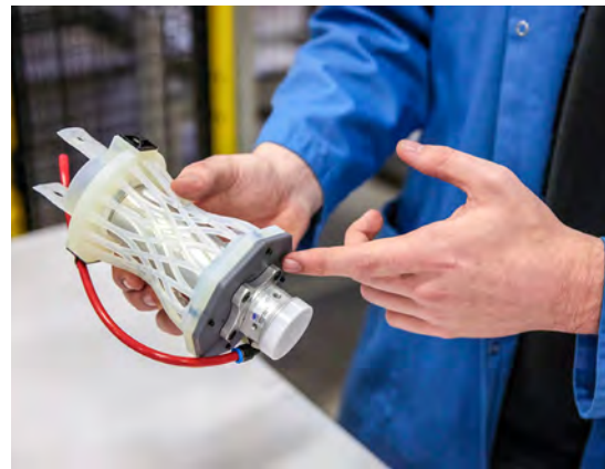
Consecutive iterations of a pick and place robot gripper prototyped on Formlabs SLA printers.
