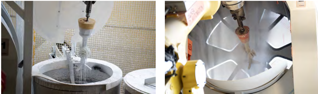
UNI's robotic cell picks the tree and dips it in the primary slurry (top), drains excess slurry at the end of the process, then inserts it into a rainfall sander (bottom).
