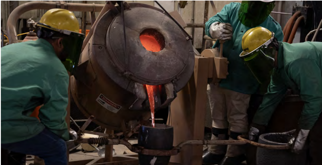
University of Northern Iowa (UNI) team pouring metal from melt furnace into a crucible
