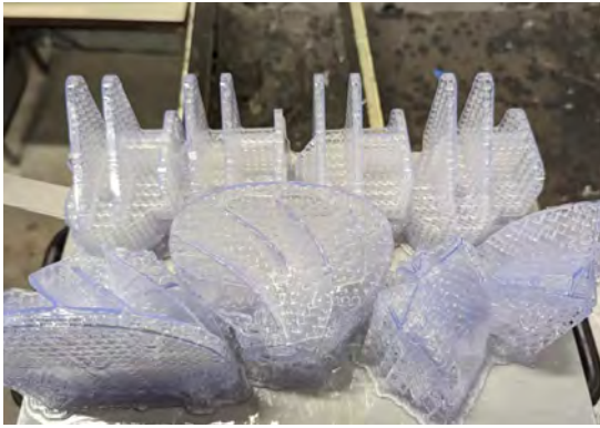
UNI's patterns on the Form 3L Build Platform after impression (top left), then the supports are removed and sanded (top right).
