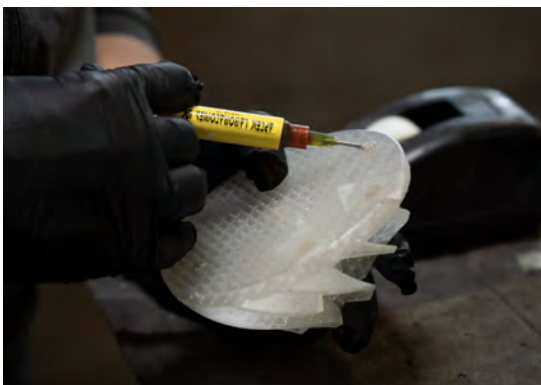
UNI's team plugs the holes with wax (left) and attaches the pattern to the tree (right) for automated investment casting using a pick-and-place robot.
