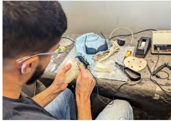
UNI's patterns on the Form 3L Build Platform after impression (top left), then the supports are removed and sanded (top right).
