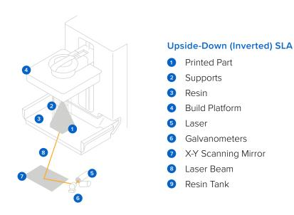
A graphic representation of the basic mechanics of stereolithography 3D printing.
