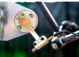
Engineers at AMRC use a fleet of 12 SLA 3D printers and a variety of engineering materials to print custom parts for diverse research projects, like brackets for a pick and place robot (left) and mounts for sensors in a high-temperature
