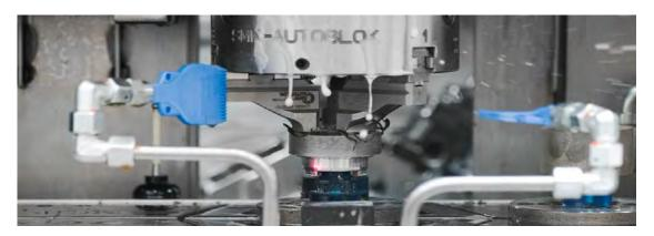
Because they are isotropic, SLA printed parts like this jig from Pankl Racing Systems can withstand the variety of directional forces they undergo during high stress manufacturing operations.
