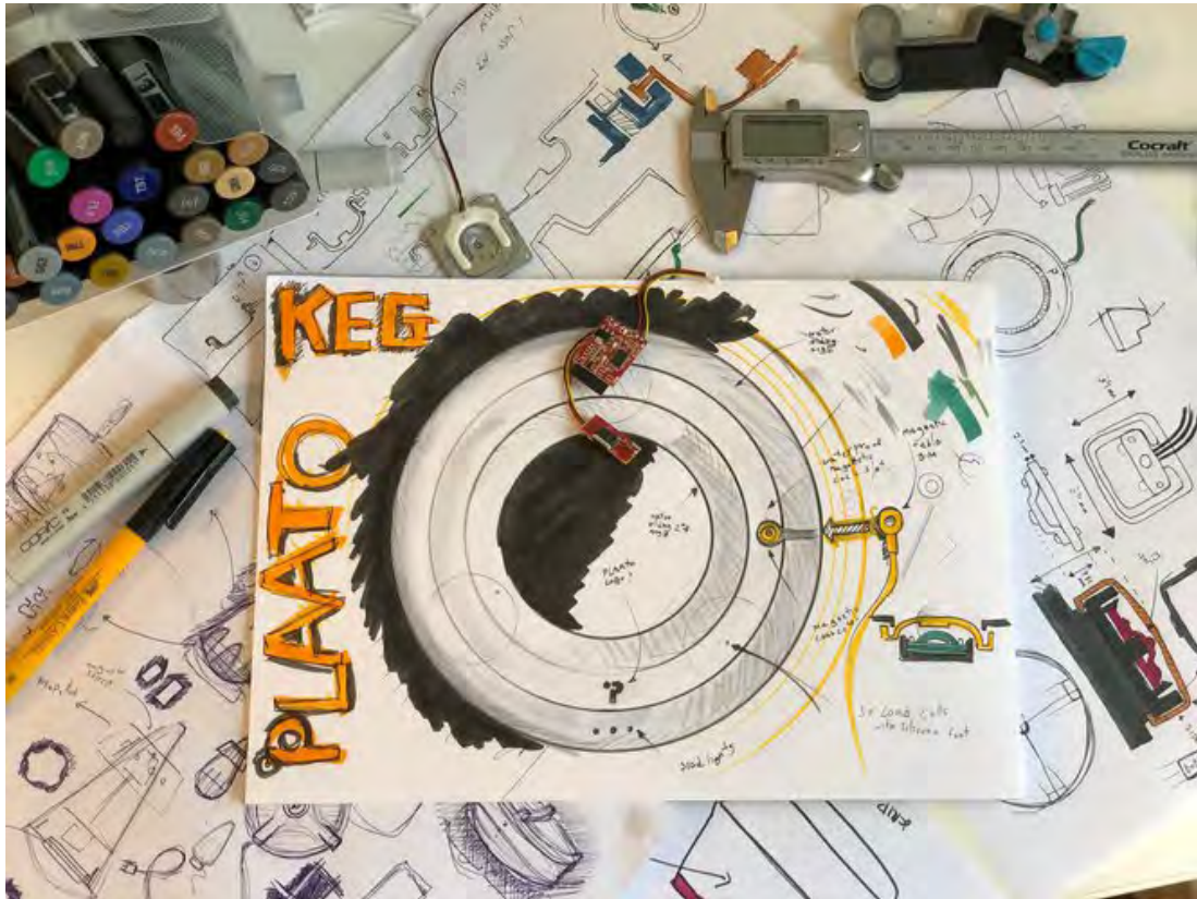
Design iterations of the Plaato Keg, including the connector and the load cells.
