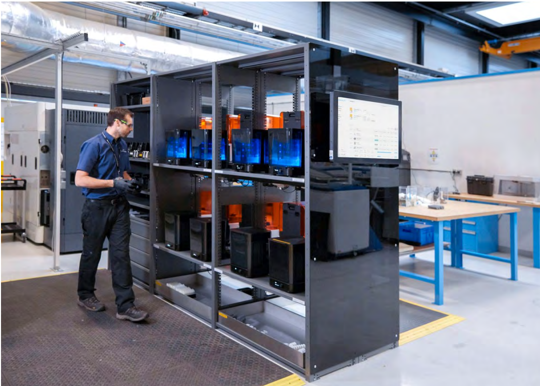
The back side of the station contains a wet area with four Form Wash and four Form Cure units for cleaning and post-curing as well as some space storage.
