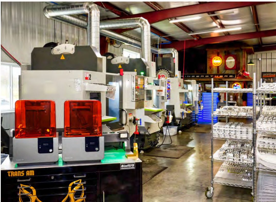
The Ringbrothers team brought SLA 3D printing in-house as a prototyping tool and have since found ways to leverage the technology to produce end-use parts.
