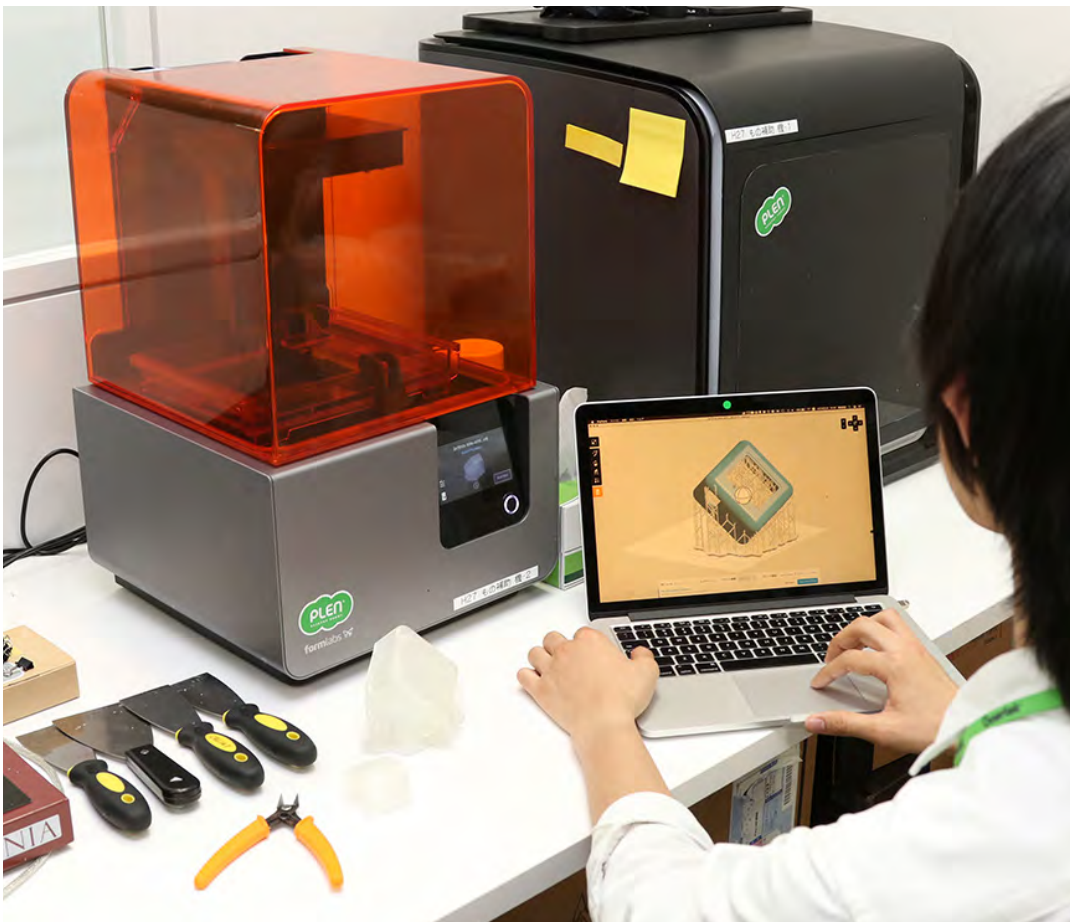
The PLENGoer Robotics team used PreForm software to optimize their prototypes before sending them to the Form 2 SLA 3D printer.
